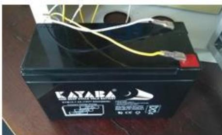
Gambar. 14. VRLA Battery
